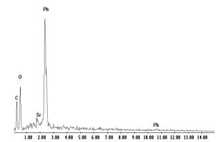
Fig. 5. PbCO<sub>3</sub> particle in ash from individual domestic furnace with EDS spectrum.
