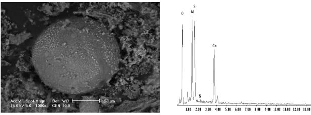
Fig. 1. SEM image with EDS spectrum of aluminosilicate particle in ash from domestic furnace.
