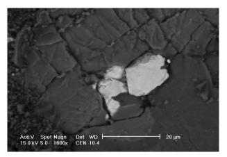
Fig. 4. Barite particles (white points) in ash from domestic furnace.
