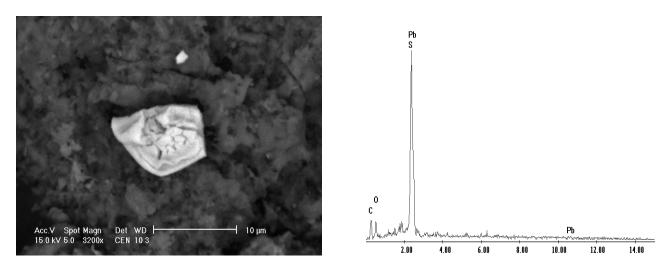
Fig. 2. SEM image with EDS spectrum of PbS in ash from individual domestic furnace.
