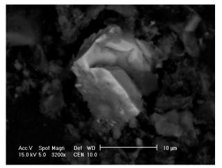
Fig. 7. SEM image of monazite particle in ash from domestic furnace.
